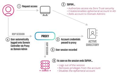
As a tier-1 component, the proxy has been designed with self-healing redundancy and the capability to scale using an architecture supported on both Windows and Linux.
